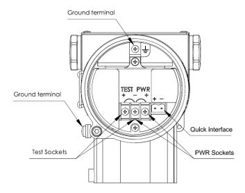
Note: Quick interface functionally equivalent to the signal terminal
