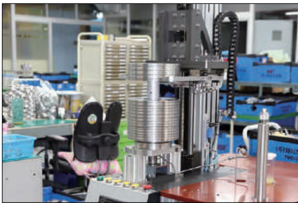
Dead-weight calibrating machine for high pressure PG
