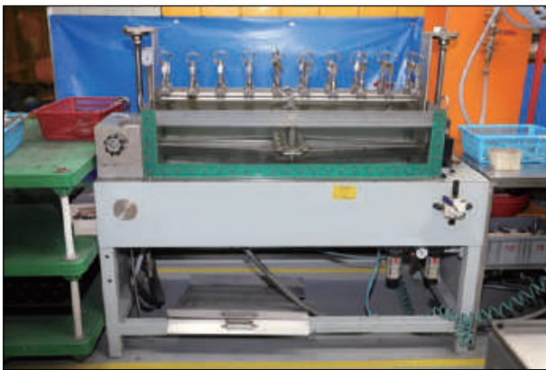
BT welding leak test machine waterlogging
