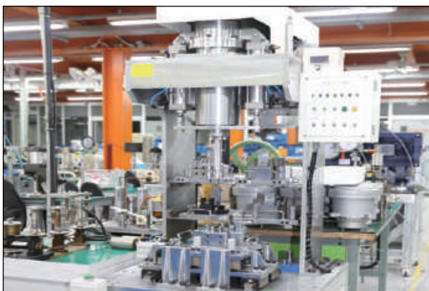
Bolt assembling machine for DP gauge
