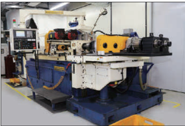
Gundrill for thermowell processing
