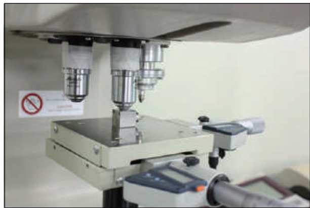
Hardness tester for pressure gauge parts
