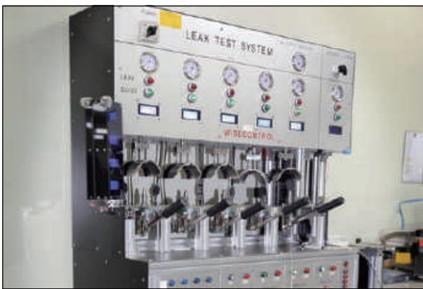
Helium leak tester for the welding area (for PG)
