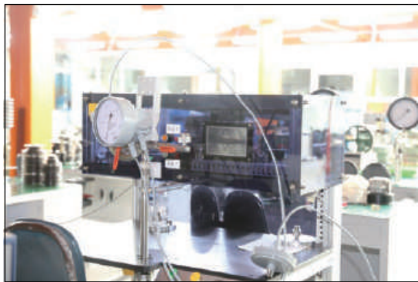
Low pressure calibration for DP gauge
