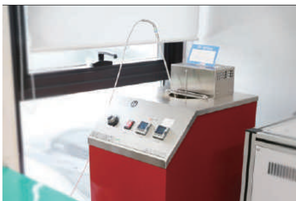
Furnace for calibrating temperature for ^{\circ}\text{C} (Below zero temperature)
