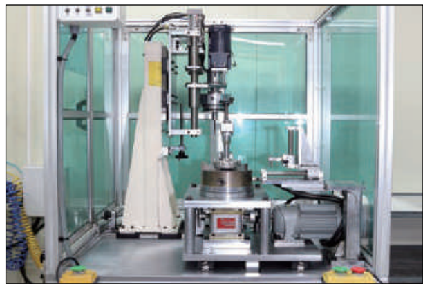
Flange bolt assembly machine for diaphragm type PG
