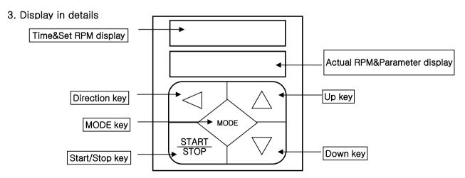
4. Function of each S/W TYPE(It could be changed by A-Type or B-Type as per each product)
