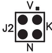
**Figure 5: Mode Programming Jumpers**
