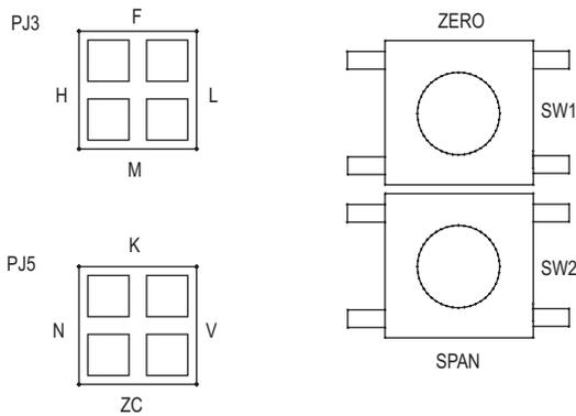
**Figure 5: Mode and Range Programming Jumpers and Switches**
