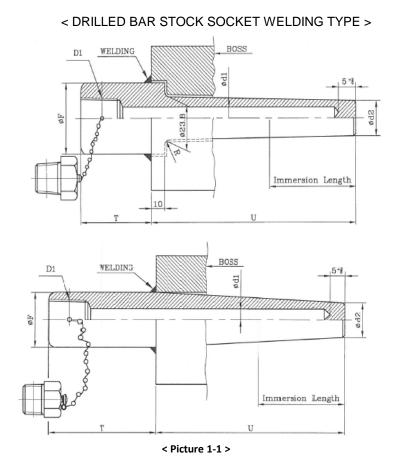
Install a Thermowell to the BOSS where want to install. (Refer to picture 1-1) After the installation, perform the tack welding around a welding point After checking install state, perform the welding if no problem.
