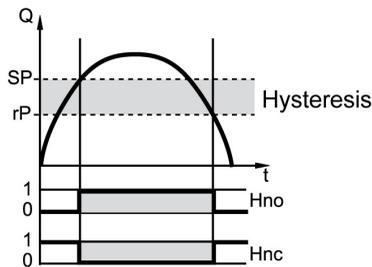
The hysteresis keeps the switch status of the output stable if the flow fluctuates around the nominal value.
