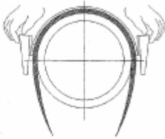
Hang the retaining bracket correctly over the screw yoke on one side.
