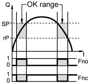
The window function allows a defined OK range to be monitored.
