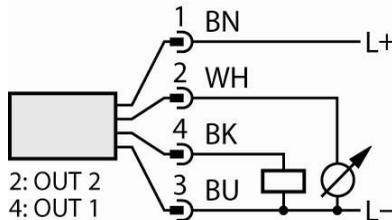
Pin assignment on the cable connector
