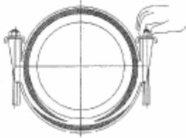
Using the wrench, rotate further until the retaining bracket slips over the screw yoke and clicks into place.
