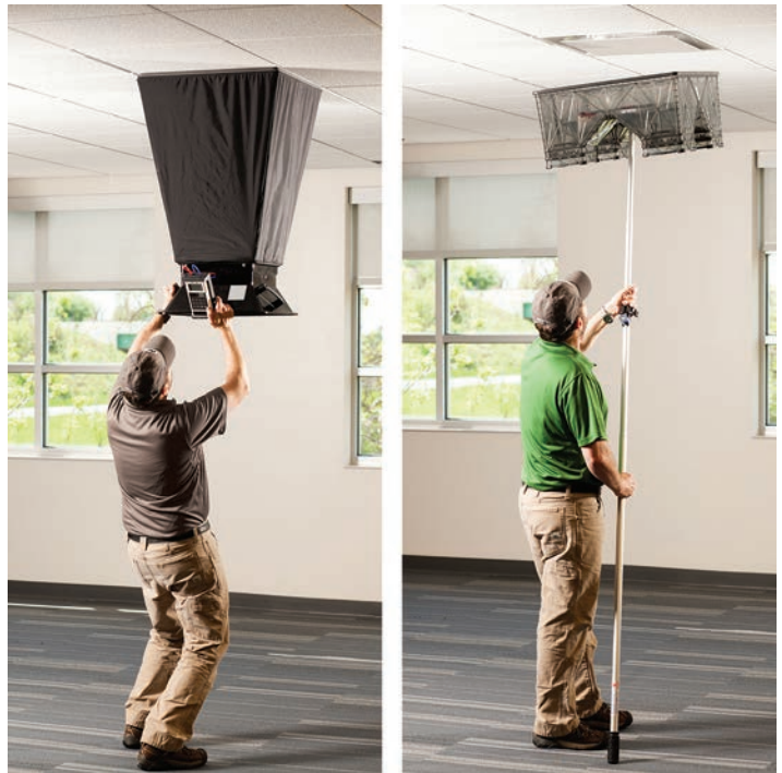
Figure 1 – Traditional Air Flow Hood (left picture) versus Dwyer Smart Air Hood (right picture)
