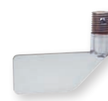
PDL-4 Minimum bulk density of 70 lb/ ft 3 (1122 kg/m 3 ). Fits through 1-1/4" coupling eliminating the need for a mounting flange.
