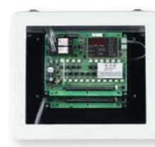
Master board stacked with channel expander
